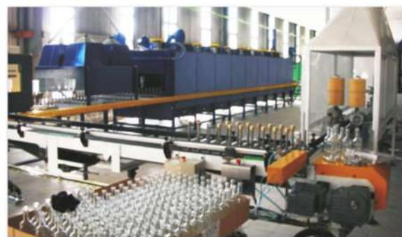
**Furnace workshop № 3:** 2 IS machines and 1 rotary glass-forming machine. Bottles for alcohol, food industries, glass jar.
